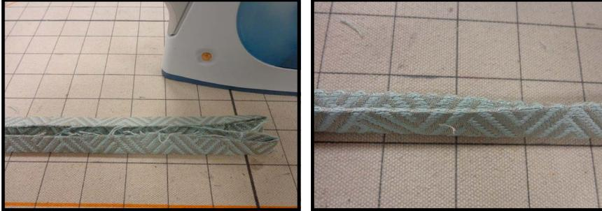
**5** On the front, glue-baste the welt to the sides and top, cutting away the welt from the casing at the start and stop points.
